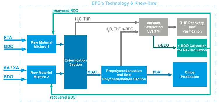
EPC's PBAT polycondensation process uses 1.4 butandiol and a combination of dicarboxylic acids as raw materials. One significant advantage is that the spent-BDO, THF and H2O are collected, treated and reused; fullfiling EPC's Circular Economy-Standard. While the liquid spent-BDO is recirculated into the process, the recovered THF can be sold to the global market as a highly valuable organic solvent.
